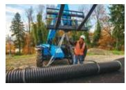
All Genie telehandlers come equipped with a lift shackle that enable you to sling a load without secondary attachments. A factory lift shackle lift chart also sets the user and safety inspectors at ease.
