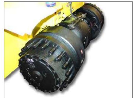
The steer axle (left) has a robust design and excels in the roughest applications. It provides a tight turning radius, as well as effortless power steering due to its double-acting cylinder, which is protected by heavy steel support beams. The planetary drive axle (above) is specifically designed for heavy-duty applications. Gear reduction at the hub reduces maintenance costs and allows a larger ratio while supporting a small differential.
