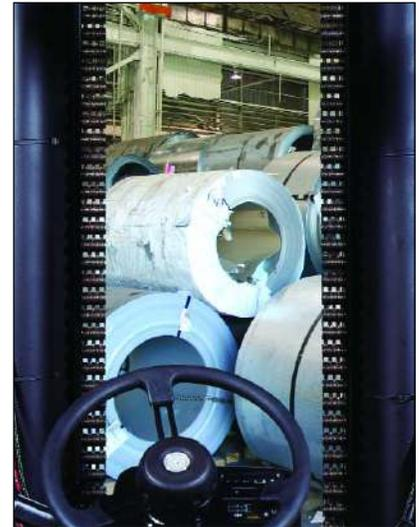
The **Lazer Series**' two-stage, hi-vis mast (optional three-stage and full-free lift mast options available) provides excellent forward visibility.
