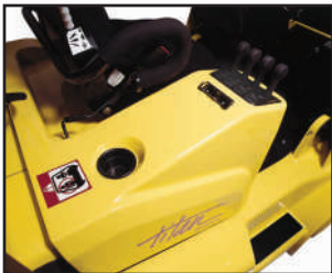
Soft-touch hydraulic levers require minimum effort. Clipboard and cup holder located by controls.
