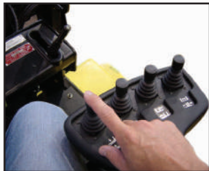
Optional finger-tip levers are designed to move within the full range of seating positions.
