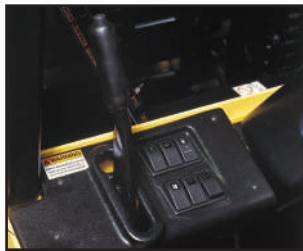
Parking brake, gauges and controls located on dashboard.
