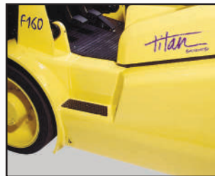
Low, 18-inch, non-skid steps for safe and easy entry and exit.
