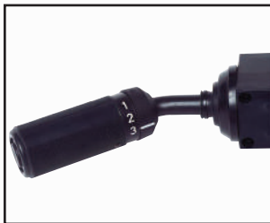
Directional/gear-shift lever located on steering column.
