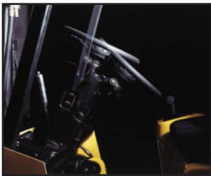
Tilt-steering column. Easy entry and exit for any size.
