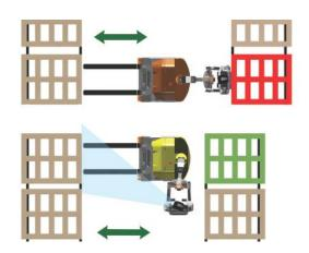
Standing to the side of the stacker eliminates the risk of being trapped or crushed whilst allowing the Combi-CS to operate in very narrow aisles.
