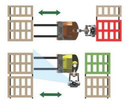
Standing to the side of the stacker eliminates the risk of being trapped or crushed whilst allowing the Combi-WR to operate in very narrow aisles.
