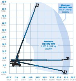
\* The metric equivalent of working height adds 2 m to platform height. U.S. adds 6 ft to platform height.
