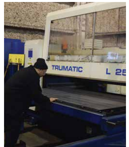
Trumpf Laser 2000 Watt, 48" x 96" L2520 for tight tolerance precision cutting with +/-0.005" accuracy for material up to 1/2" thick.
