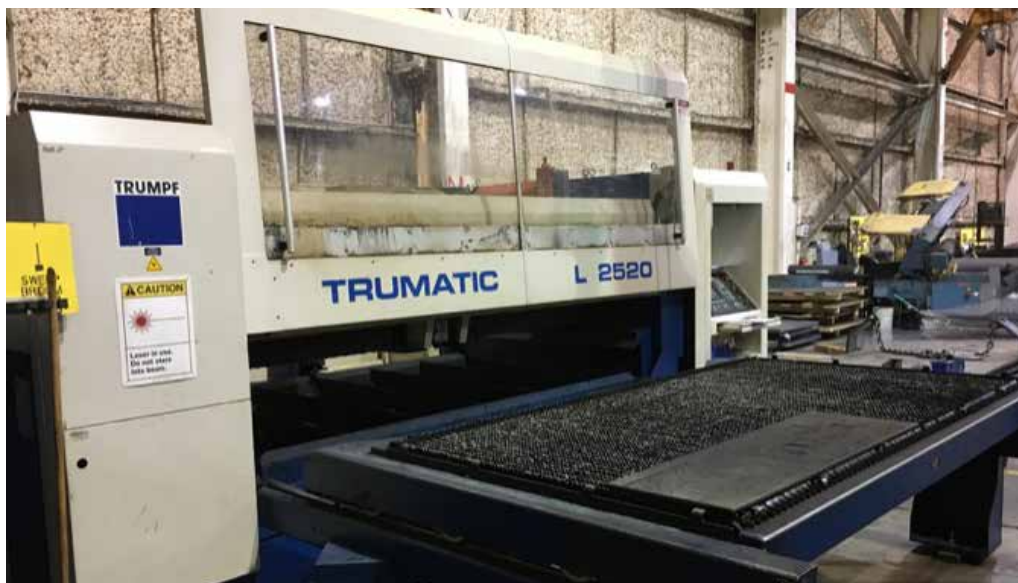
Trumpf Laser 2000 Watt, 48" x 96" L2520 for tight tolerance precision cutting with +/-0.005" accuracy for material up to 1/2" thick.
