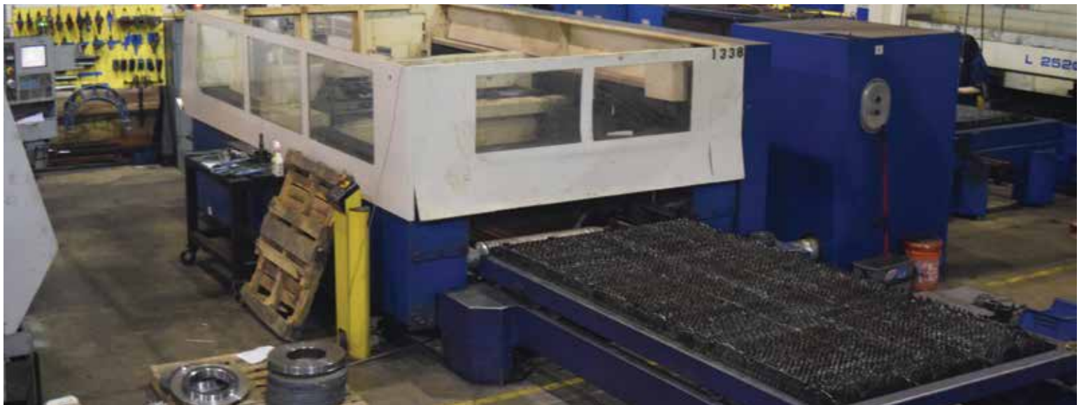
Trumpf Laser 4000 Watt, 60" x 120" TLF 4000 Turbo for tight tolerance precision cutting with +/-0.005" accuracy for material up to 3/4" thick.
