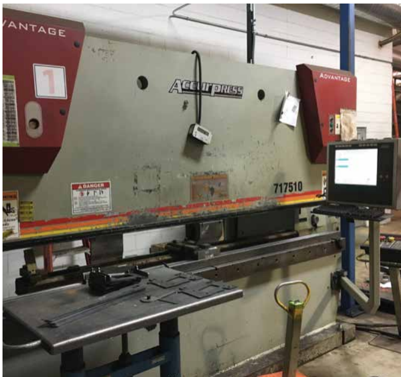
Accurpress 175 Ton full CNC control Press Brake X 120" long utilizing the latest in high-speed precision bending technology.
