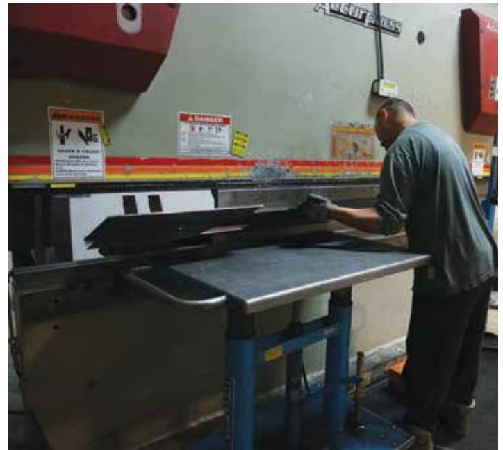
Accurpress 175 Ton full CNC control Press Brake X 120" long utilizing the latest in high-speed precision bending technology.
