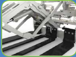
Adjustable outer platens to handle slipsheets
