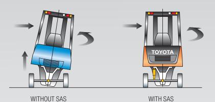
When it senses instability, > SAS instantly engages the Swing Lock Cylinder to stabilize the rear axle, creating the lateral stability needed to help reduce the risk of lateral tipovers.
