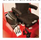
Forward facing driving position with 'clear vision' mast for safe operation. All controls biased to the right side make for easy operation.
