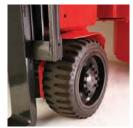
Four large cushion rubber tires deliver optimum performance and traction. They're also resistant to damage which means a long service life and less downtime.
