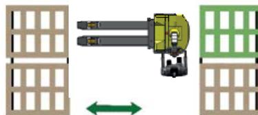
Standing to the side of the truck eliminates the risk of being trapped or crushed while allowing the Combi - PPT to operate in very narrow aisles.
