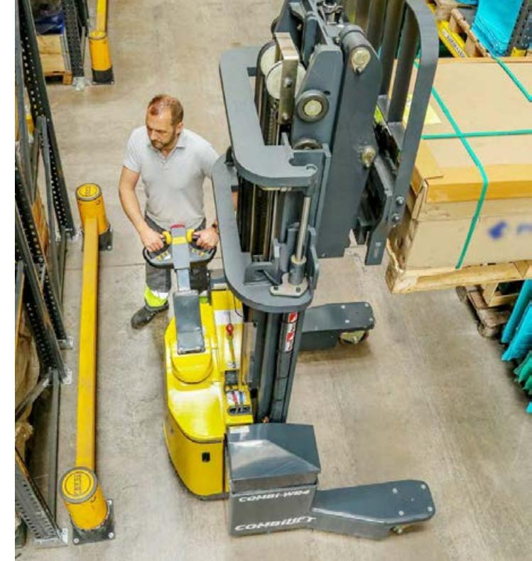
**Multi-Position Tiller Arm can be turned to the left or right, allowing the operator to stand to either side, providing full visibility of the load and forks while maintaining full steering control**
