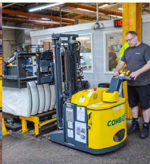
*This pedestrian reach stacker can operate in the narrowest aisles of any truck of its type in the market.*
