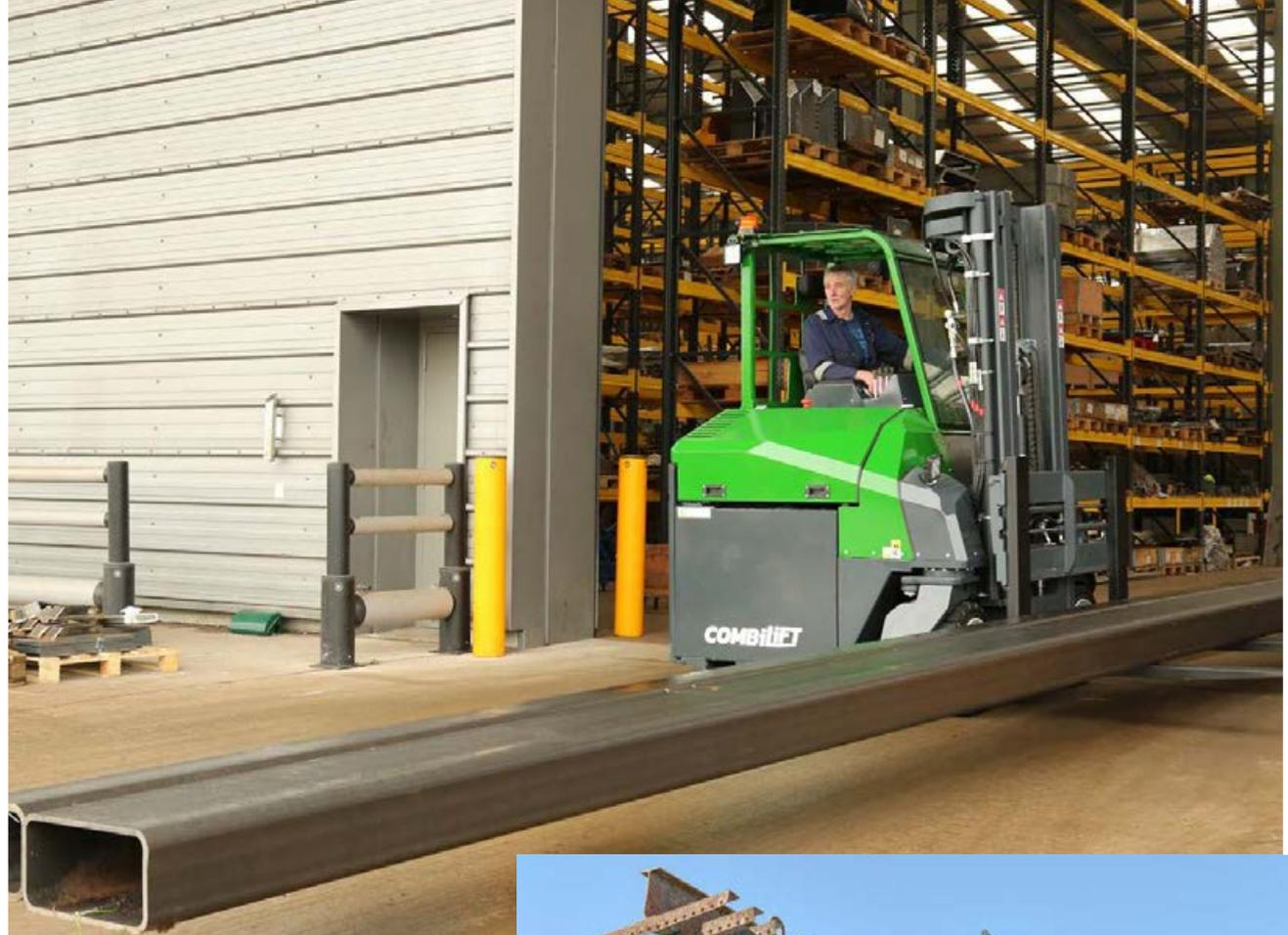
*Counterbalance operation combined with the ability to carry long loads, such as timber or steel beams, in sideways mode makes the COMBi-CB the most versatile all-round forklift available.*
