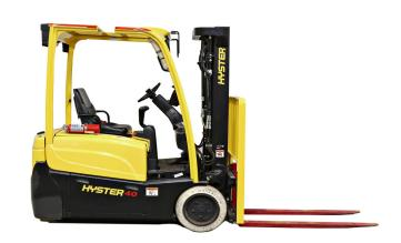
Active Mast Control monitors lift height and load weight, automatically reacting to limit or prevent tilt and reduce the likelihood of a tip over.
