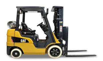
System of Active Stability™ and Active Mast Control™ monitor forklift conditions and automatically reacts to reduce the likelihood of a tip-over when traveling and load handling
