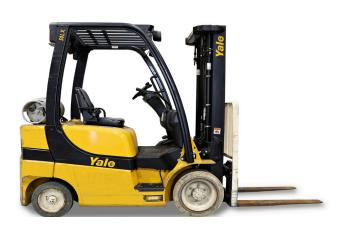
System of Active Stability™ and Active Mast Control™ monitor forklift conditions and automatically reacts to reduce the likelihood of a tip-over when traveling and load handling
