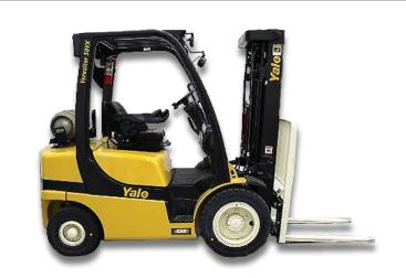
System of Active Stability™ and Active Mast Control™ dynamically monitor forklift conditions and automatically reacts to reduce the likelihood of a tip-over when traveling and load handling
