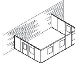
2-Wall and 3-Wall buildings utilize your existing walls and minimize cost. Steel roof deck adaption is provided for support at existing walls.
