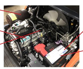
If not a maintenance-free battery, is the water at the correct level? (Visual)
