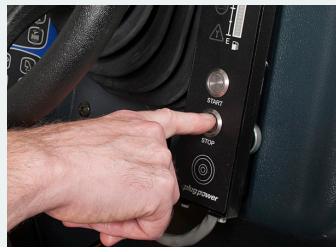
2 Turn the Fuel Cell off by pushing the STOP button
