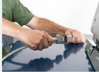
Connect fuel cell to controller
