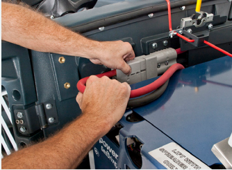
Connect fuel cell to CS7010 unit
