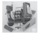
The SW4000™ offers MaxAccess with tools-free side cover removal for full access to the battery compartment and main broom drive components.
