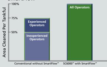
SmartFlow™ adjusts solution flow with the machine's speed, using up to 50% less water and chemicals. Proportionally higher productivity with fewer dump and refill cycles per tankful.
