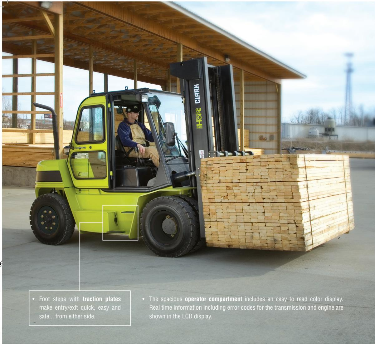
• Foot steps with traction plates make entry/exit quick, easy and safe... from either side.
