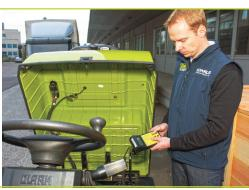
• The CLARK handset can be used for diagnostics and settings of up to 20 different performance parameters to match your requirements.
