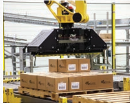
Robotic Palletizer and Depalletizing Systems
