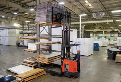
With **Auto Height Select**, the operator can select up to 25 programmable present lift heights, using the reach and retract control handles buttons. When the operator lifts, the carriage stops automatically near the selected height. The operator then finely adjusts the height manually to place the load in the rack location.
