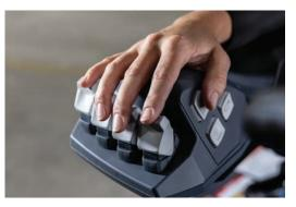
**Toyota's EZ Control Joystick**<sup>®</sup> offers a progressive, ergonomic approach to material handling by putting all hydraulic controls, horn button, and travel direction in a singular handle. An intuitive axis-based pivot combined with strategic button placement and smooth operation puts operators comfortably in control of the most precise material handling challenges. The ergonomic design helps reduce operator fatigue and allows for multiple functions at once such as lift and tilt.
