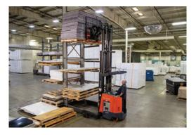
With **Auto Height Select**, the operator can select up to 25 programmable present lift heights, using the reach and retract control handles buttons. When the operator lifts, the carriage stops automatically near the selected height. The operator then finely adjusts the height manually to place the load in the rack location.
