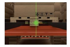
**Toyota's Acu-Laser** automatically projects a red or green laser line onto the pallet, allowing precise pallet placement and showing the operator the the fork's position.
