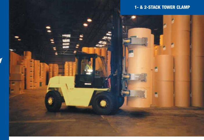
A durable paper roll clamp for handling two to eight rolls in high-cycle operations.
