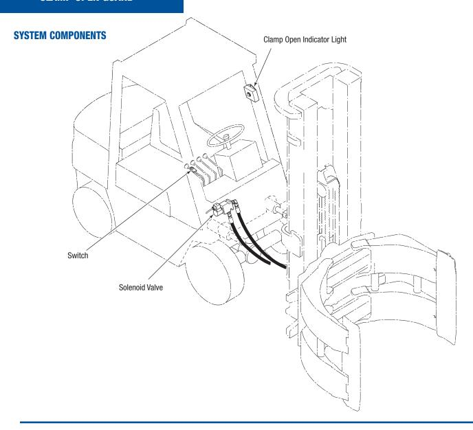
The Clamp Open Guard will require the driver to hold the button down while opening the arms.
