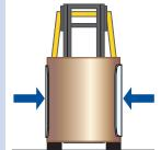
Computer-based clamping systems that automatically control the clamp force in proportion to the load weight.
