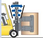
Automatically controls the angle of the mast and attachment, aligning pad with the load.
