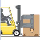
The Clamp Open Guard system automatically prevents the roll from being unclamped while it is lifted.
