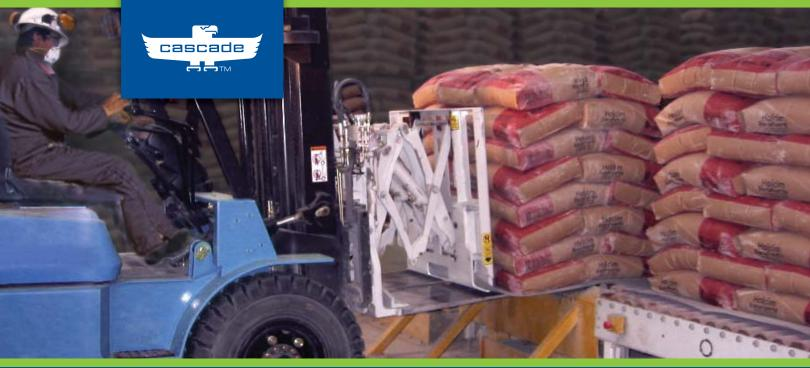
Pallet-Free Cement Handling with Heavy Duty Push/Pulls from Cascade.
